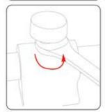
**NOTE:** the main (large) screw needs to be tightened in to position before the grub screw.
